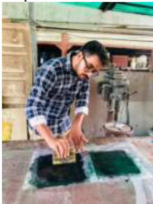
Fig 1: hand lay up technique.
